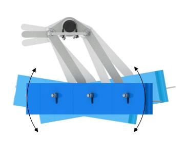
Adjustment of the angle for the distribution of the blade pressure between the center and the sides
