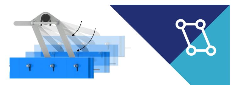
The articulated parallelogram support keeps permanent contact with the belt regardless the level of wear of the blade and allows it to rise-up in dangerous situation
