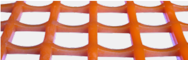
Poliuflex® screen Aperture 9 thread 4 mm after 1150 hours carrying out wet screening of quartzite material with 97% SiO 2
